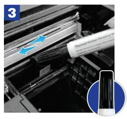
If needed, Use scraper cap to remove stubborn buildup
