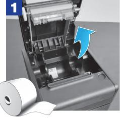
Turn off printer, open, and remove media roll
